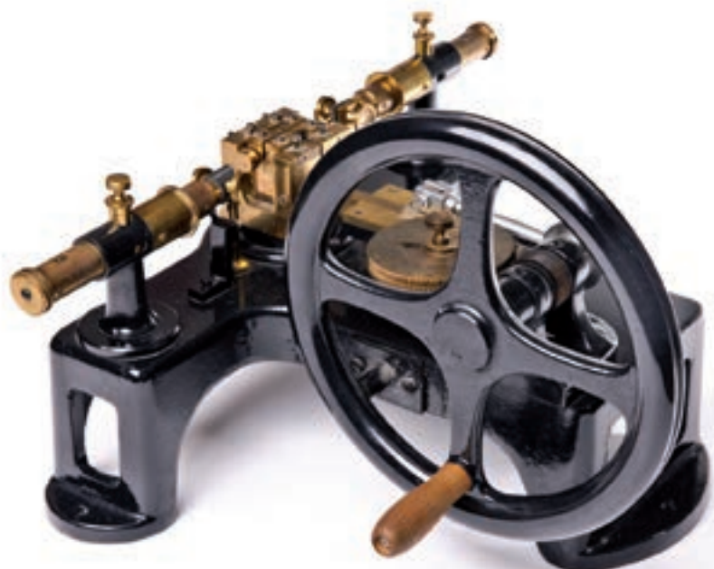
Devices examining the resistance to double folding from ca. 1920 (collections of the Museum of Papermaking, sign. MD 49 T)
